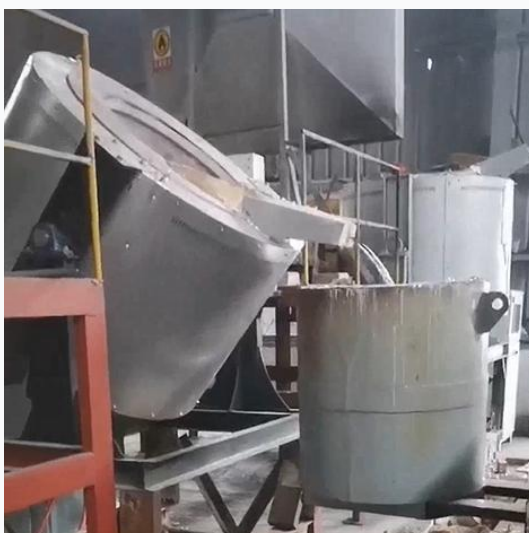
1Ton Al tilting furnace *1 sets
