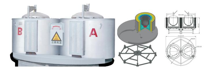
This furnace is specifically designed for advanced aluminum alloy melting and holding, suitable for low-pressure casting and liquid forging processes. The base is equipped with a motor and reducer, allowing it to rotate 180 degrees to the desired position for robotic arms.
